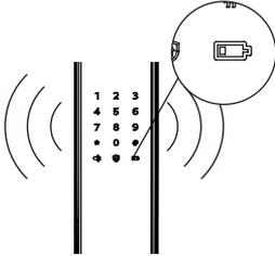
**Way to trigger:** When the system wakes up, it will automatically check the battery voltage. If the voltage is too low, then an alert will be triggered to remind you to replace the batteries.
