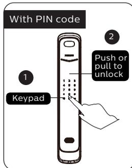
① Touch the digit input area to light up the keypad and enter the registered PIN code and confirm with [#].
