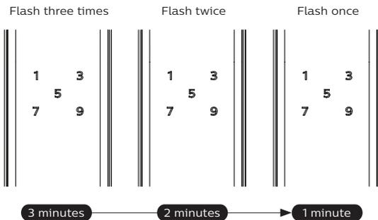
If there are consecutive incorrect inputs of any of the fingerprint, PIN code, or key tag 5 times within 5 minutes, the system will lock up for 3 minutes.
