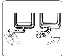
③ Make a 180 degrees twist clockwise and make sure the key shell is parallel to the horizontal plane. Then rotate the key cover horizontally in the direction of the handle to unlock.
