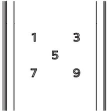
When the door is under inside deadlock mode, the keypad will lock. If you wake up the system manually, the keypad will show the combination of "15937 (X)" with a voice prompt of "inside deadlock enabled".
