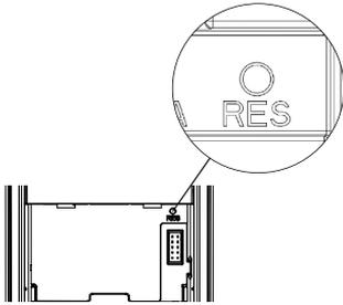
Remove the battery cover, then double press the [RES] hole with a sharp object. When you hear a voice prompt of "Restoring to default settings", it means all user record is emptied.
