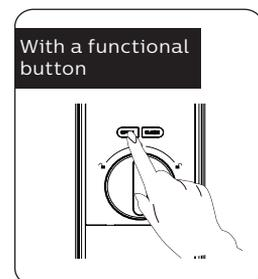
Double press the [OPEN] functional button within one second, then push or pull to unlock the door.
