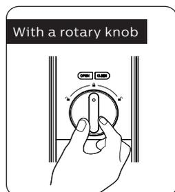
Philips EasyKey adopts indoor fast opening mortise. You can unlock the door from inside by rotating the rotary knob.
