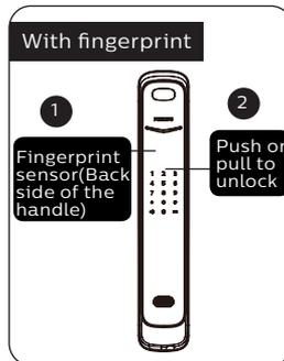
① Place the registered finger on the fingerprint sensor.
