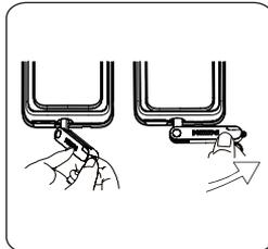
② Insert the key into the keyhole and the key should be vertical to the key shell. Then turn the key shell by 90° in the direction of the handle until it is close to the lock.
