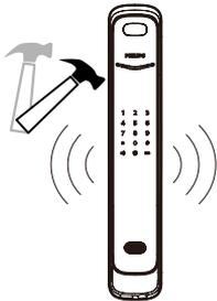
**1. Way to trigger:** The door is pried apart and the latch bolt is popped up.
