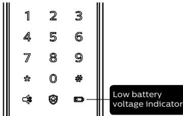
**Red:** When the system wakes up, it will automatically check the battery voltage. If the voltage is too low, then the light will flash in red and there will be a voice prompt of "Low battery voltage, please replace all batteries".
