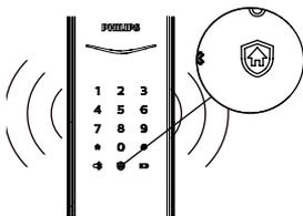
**Way to trigger:** Upon enabling the outside deadlock mode, an alert will be triggered when you unlock the door from inside.
