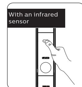
Philips Easykey has an infrared sensor on the handle. When the sensor is triggered, you can press the sensor module on both the front and rear sides of the handle simultaneously to unlock the door.
