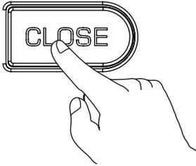
When the EasyKey is locked, long press the [CLOSE] button until the indicator flashes once in red, then there will be a voice prompt of "Inside deadlock enabled".
