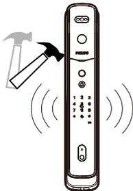
**Triggering 1:** The door is pried open, and the sensor latch bolt pops up.
