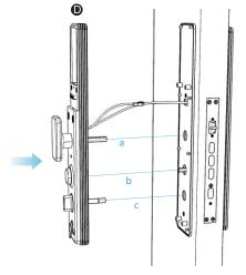
② After ensuring a, b, c are all in right positions, fix "D" on the fixed plate.
