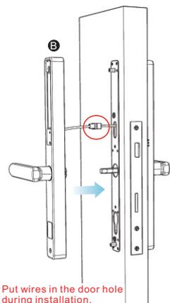
Put wires in the door hole during installation.
